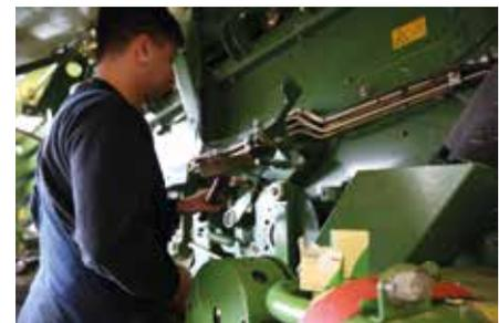
Willy Pripke, one of Marep's fitters, installing the new connecting rod
